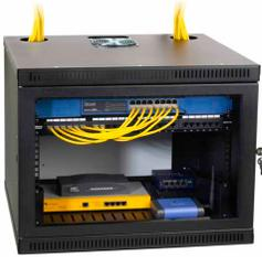
**A Network Box** – Stores normally have a box or place near the back where the internet equipment is set up. You’ll see a router, a switch, access points, and other devices used for networking in this box. Find yours.
